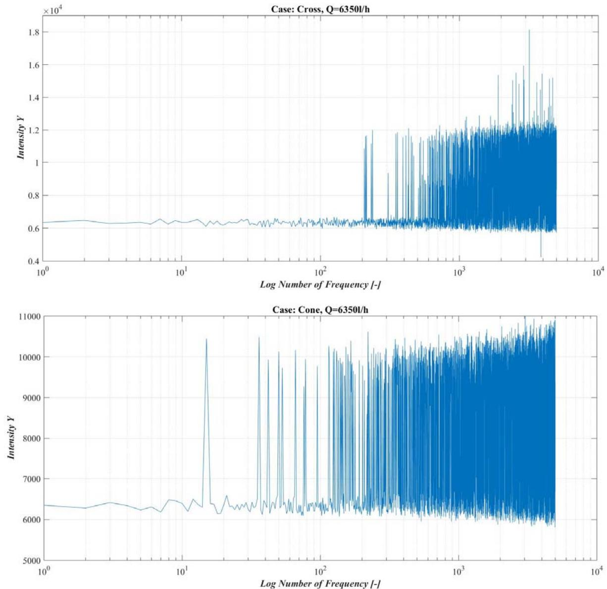
Figure 2 FFT Spectrum of the 5,000 most prominent pre-processed frequencies for the obstacles Cross (top) and Cone (bottom) at 6350  $l/h^{-1}$  in semi logarithmic scale.
