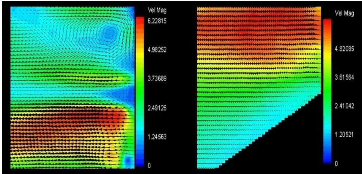
Figure 1 Processed PIV images on a normalised scale for the obstacle types “cross” (left) and “cone” (right) at 6,350  $lh^{-1}$
