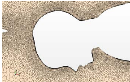
Fig 3 Computational grid around a streamline model
