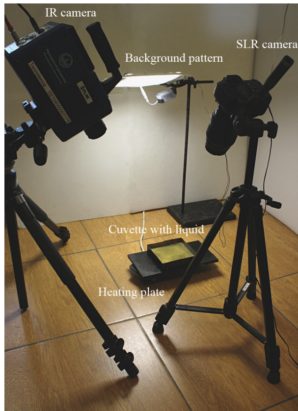
Fig. 5 Experimental setup for simultaneous measurements of surface deformation and surface temperature fields.
