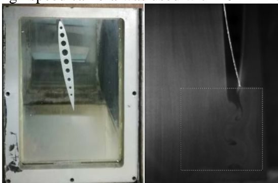
Fig. 4 NACA0012 airfoil Model and particle image
