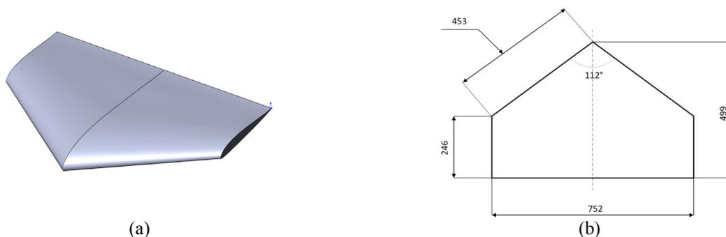
Fig.1. Flying wing (a) and its parameters in mm (b)
